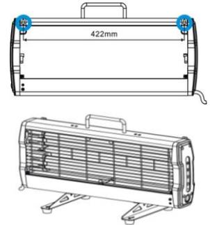
\* When using by Wall Mounting, the device should be installed with the Reflector. When using by Floor Standing, the device can be installed with the Reflector if it is placed against wall, or without Reflector if it is placed away from wall.
